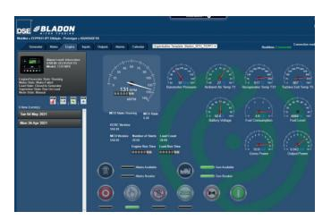
Also equipped is a Deepsea DSE890 MKII Gateway unit and built-in antenna, which can be connected to the internet for remote monitoring and remote control:
