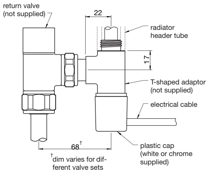
The IHE electric heater should be fitted vertically through the 'T' shaped adaptor (not supplied) and installed on the return side. (See illustration).
