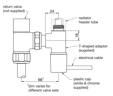
The DE-PACK electric heater should be fitted vertically through the 'T' shaped adaptor supplied and installed on the return side. (See illustration).
