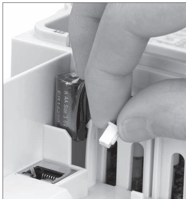
Figure 1. RTC battery connection
