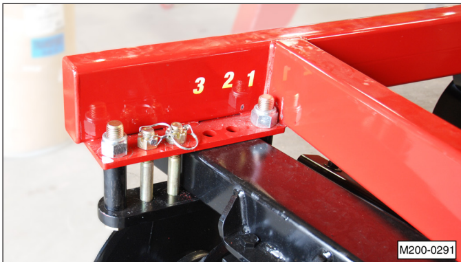
Adjustments for front disk gang.
