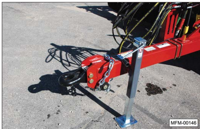
Transport lock secured in storage position.
