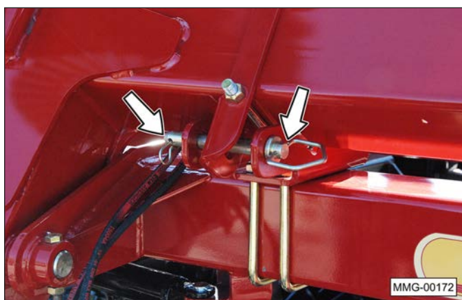
Transport lock secured over cylinder rod.
