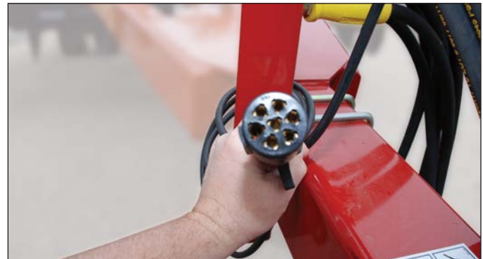
d. Connect the plug into the tractor's electrical socket.
