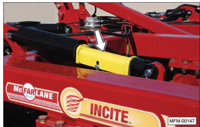
Transport lock secured over cylinder rod.
