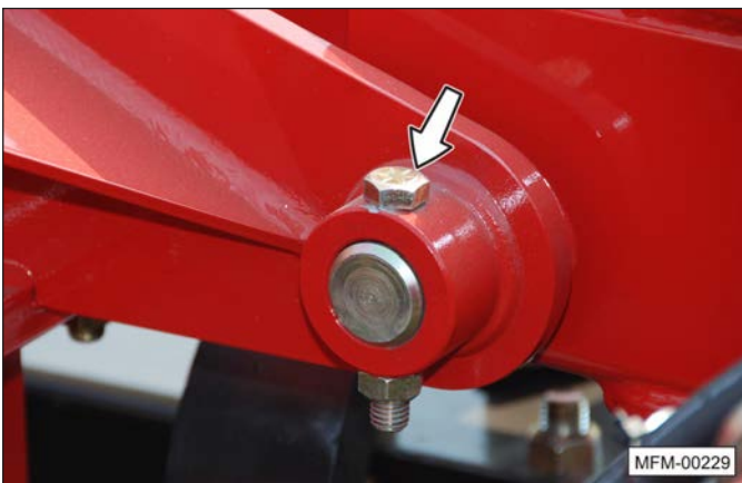
Hinge pin and hitch pin retainer bolts.
