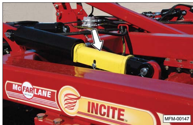
Transport lock secured over cylinder rod.
