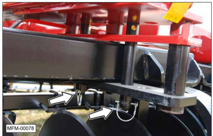
Retainer pins with wire retainer clips.
