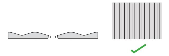
• For double height installations, trim the top and bottom of the panels with a straight blade at 90° to the panel to remove the bevel edge. Removing this slight scalloped effect from the ends will result in a smoother join
