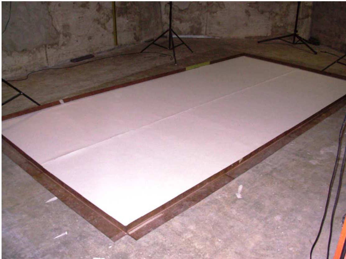
Figure 1: 2mm EchoPanel Wall installed for testing in the Reverberation Chamber.
