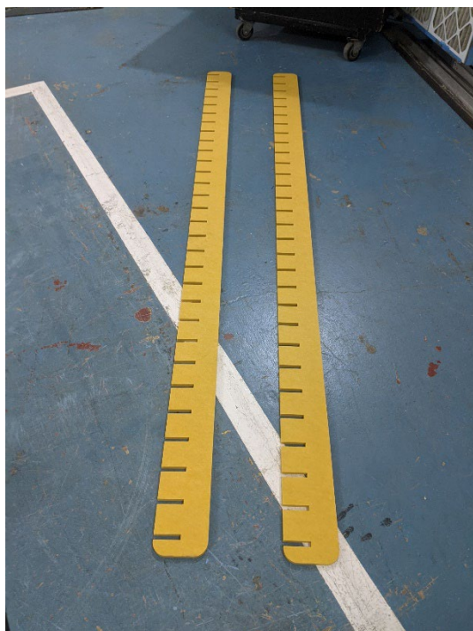
Figure 3 – Specimen pair of channels prior to assembly into baffle
