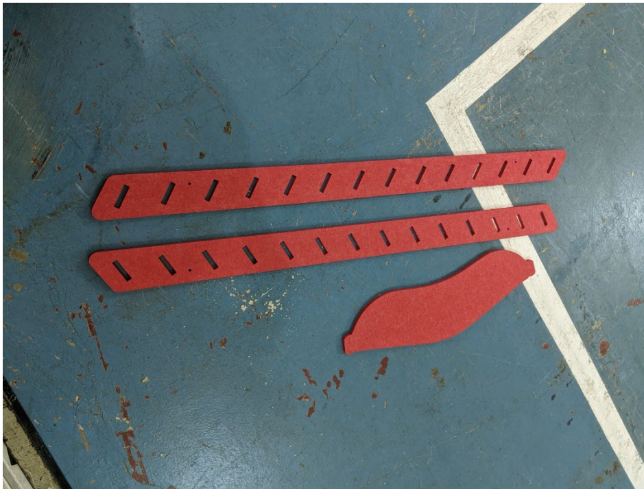
Figure 3 – Specimen fin and pair of channels prior to assembly into baffle
