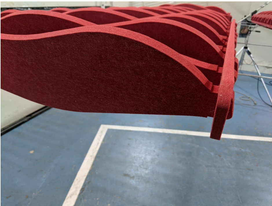
Figure 4 – Detail of assembled baffle in test chamber
