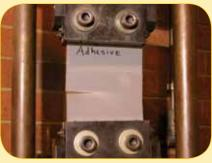
ADHESIVE AFTER: Adhesive after pull test. Adhesive at 2" overlap, metal tears at an average of 13,260 lbs. (joint did not break).
