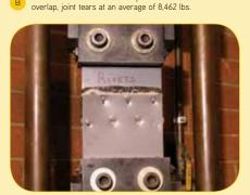
RIVETS AFTER: Rivets after pull test. Rivets at 3.5"
