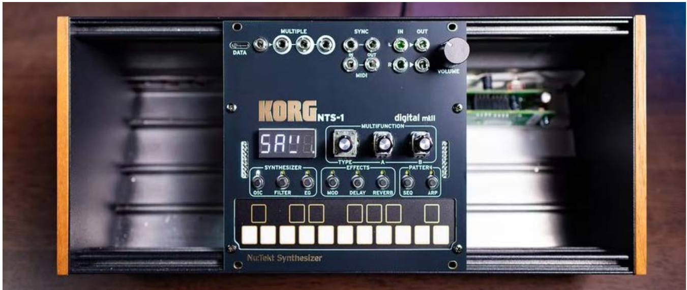
NTS-1 Mk2 Eurorack Conversion Kit. Installed and ready to patch.
