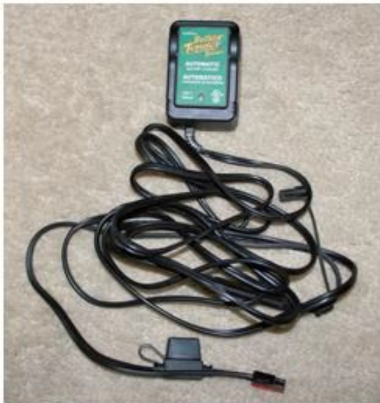
Deltran Battery Tender Junior Model 021-0123 Input – 120 VAC Output - 12V at 750 mA
