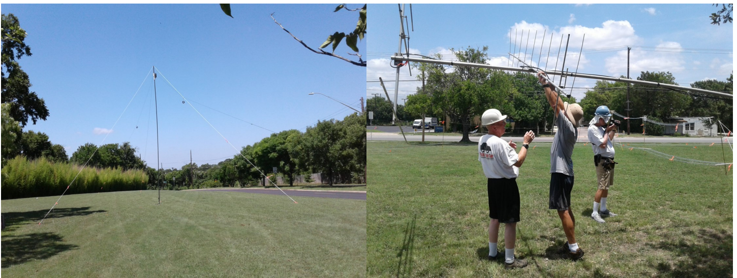
Hard to see in the pic, but bright ribbons mark the antenna wires and guy ropes of this inverted Vee.
