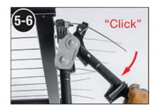
Close the handles smoothly to tension cable. An audible "click" and a slight kickback at the handles indicates the selected tension has been applied to the cable.
