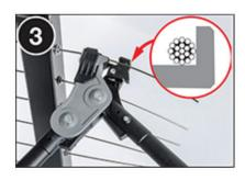
Spread handles and insert cable into the tool. Confirm that the cable is fully seated in the channel at the gripper jaw.
