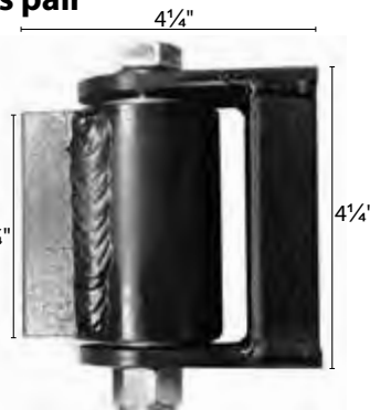
HDRBH4 4" Hinge Sealed Bearing (1.849 O.D. x .786 I.D. x .550 Thick) 5" \frac{5}{8} Bolt with nylock self-locking nut 220 Degree swing 1700 lbs/pr capacity
