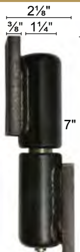
BRHS7-8 7" Steel with \frac{3}{4} " SS pin 1 \frac{1}{2} " major dia. 900 lbs/pr capacity
