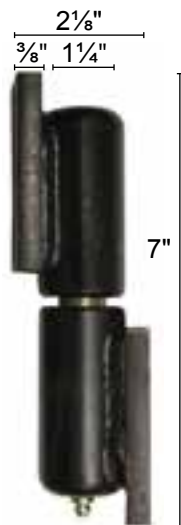
BRHS7-8 7" Cold Rolled Carbon Steel with \frac{3}{4} " SS pin 1 \frac{1}{2} " major diameter 900 lbs/pr capacity
