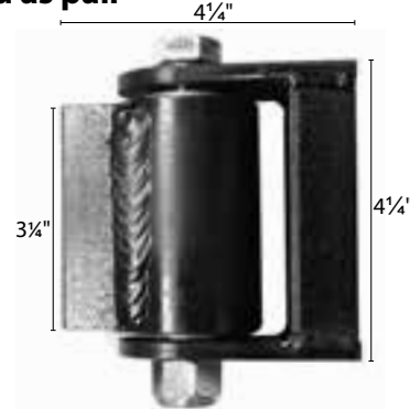
HDRBH-4 4" Hinge Sealed Bearing (1.849 O.D. x .786 I.D. x .550 Thick) 5" \frac{3}{4} Bolt with nylock self-locking nut 220 Degree swing 1700 lbs/pr capacity
