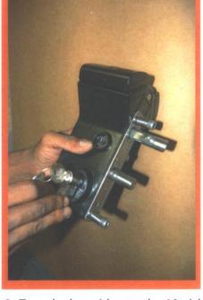
2. Turn the key either to the 10 o'clock or 2 o'clock position and slide the cylinder out of the lock body.
