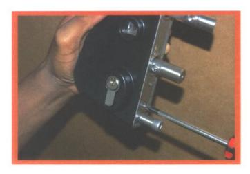
1. Remove the double cylinder dead bolt by removing the Phillips screw in the face of the lock.
