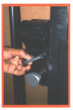
4. Install the half keyway with the plug on the "free exit" side of the gate.
