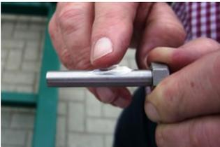
Fig. 4 Hexagon Headed Securing Pins
