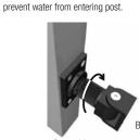
Rotate hinge onto Bracket.
