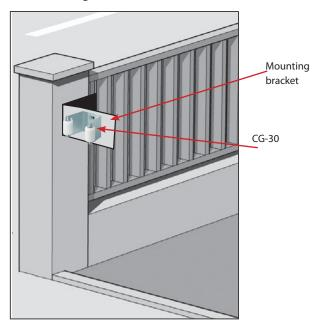
USE: Adjustable striker plate for sliding or self-supporting gates.
