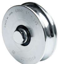
315-100 • 4" heavy duty wheel with double bearing • M14 x 70mm wheel pin • 935 lb. capacity per wheel
