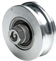
324-100 (C-44) • 4" heavy duty wheel with double bearing • M18 x 70mm wheel pin • 1278 lb. capacity per wheel • grease zerks fittings in axle
