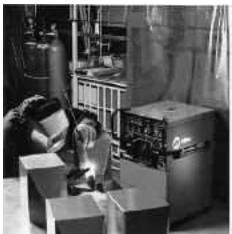
No matter what position the weld is in, thin sheet metal containers are easily welded with the pulsing feature of an industrial TIG welding machine. (Photo courtesy of Lincoln Electric Co.)
