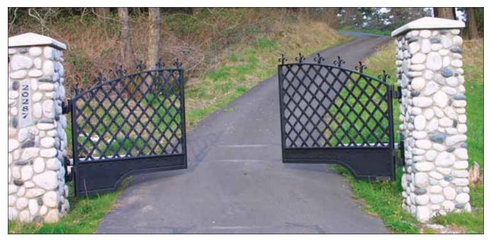
ABOVE: Cutouts at the bottom of this gate allow adequate clearance when the gate opens to the uphill side.
