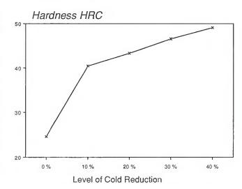
Fig. 2 — Base metal hardness as a function of percent cold reduction
