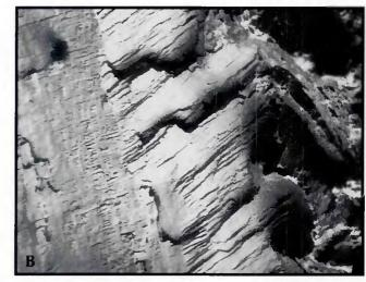
Fig. 6 — Scanning electron micrographs of a side bend fracture surface,  $2\frac{1}{2}$ T bend radius, GTA welded  $\frac{1}{2}$ -in. (12.5-mm) thick plate. A — 50X; B — 500X.
