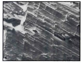
Fig. 7 — Scanning electron micrographs of tensile test fracture surfaces. Annealed base material. 5000X magnification. A — Tensile cross head speed: 10 in./min (250 mm/min), resulting in 30% reduction in area; B — tensile cross head speed: 0.001 in./min (0.025 mm/min), resulting in 18% reduction in area
