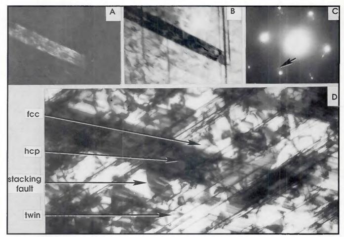
Fig. 8 — Transmission electron microscopy of UNS R31233 weld metal, 0.75-in. (19-mm) thick GMA welded plate (short circuiting transfer). A and B — Darkfield and bright-field micrographs (37,900 X) of HCP phase; C — corresponding [011] diffraction pattern. HCP streaking indicated by arrow. D — TEM micrograph (75,800X) showing FCC, HCP stacking faults and twins in as-deposited weld metal
