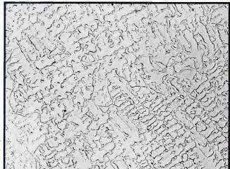
Fig. 5 — Typical weld metal microstructure (UNS R31233). GMAW deposit, short circuiting transfer. 500X magnification. HCl and oxalic etch.
