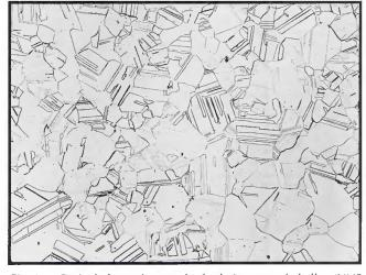
Fig. 1 — Optical photomicrograph of solution annealed alloy (UNS R31233). Magnification 300X. Hydrochloric acid and oxalic acid etch.
