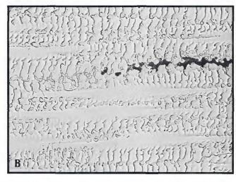
Fig. 4 — Photomicrographs of a fusion zone hot crack induced by the Varestraint test. HCl and oxalic etch. A — 100X; B — 500X, crack tip.
