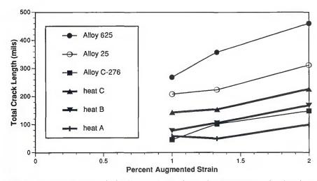
Fig. 3 — Varestraint test results for three production heats of UNS R31233. Each value plotted is an average of three tests.
