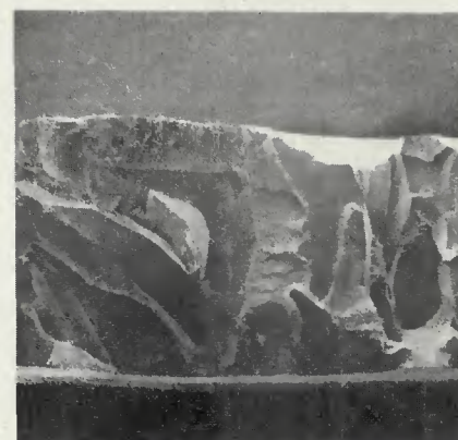
Fig. 3—Scanning electron microscope fractographs of Ti-5524S fusion zone. Tensile samples: top—as-welded, (X20, X200); middle—1400° F (760° C) /16h + 1100° F (594° C) /2h, (X20, X200); bottom—1600° F (870° C) /16h + 1100° F (594° C) /2h, (X20, X200)
