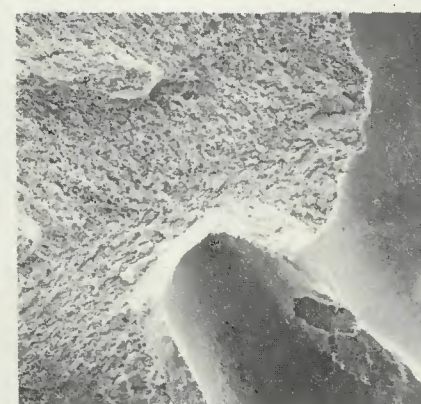
Fig. 3—Scanning electron microscope fractographs of Ti-5524S fusion zone. Tensile samples: top—as-welded, (X20, X200); middle—1400° F (760° C) /16h + 1100° F (594° C) /2h, (X20, X200); bottom—1600° F (870° C) /16h + 1100° F (594° C) /2h, (X20, X200)
