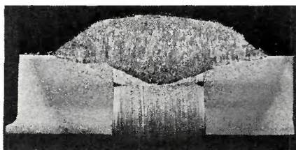
Fig. 3—Transverse section of weld bead on implant specimen showing notch location. Cracking arrested by removal of load. X5 (reduced 50% on reproduction)
