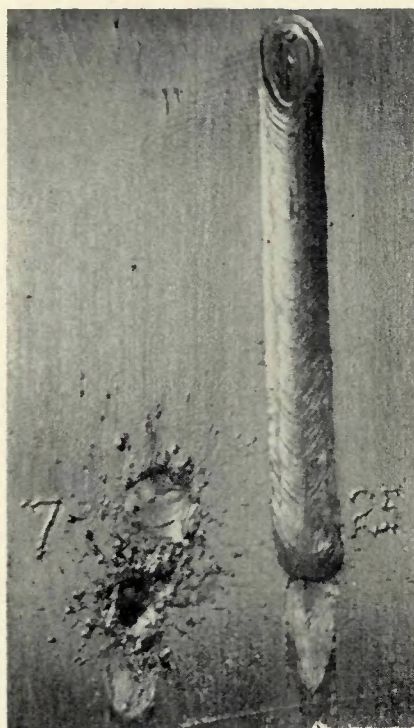
Fig. 4—Example of poor weld rated 1 and good weld rated 5
