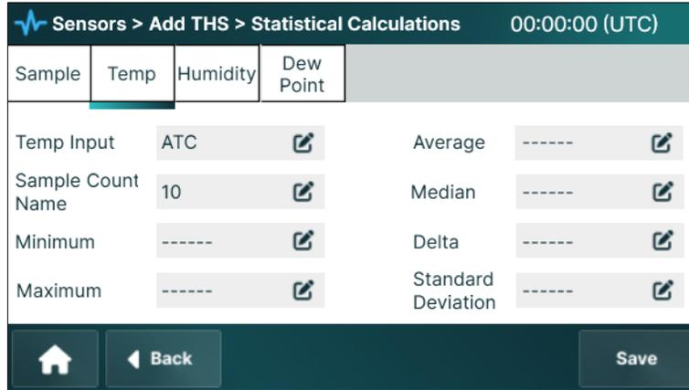
1. **Temp Input** is the sensor name to be used for the calculations.
