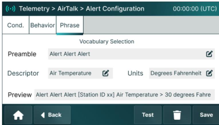
1. *Preamble* can be used to differentiate automatic Alerts from a requested Message, calling attention to a critical condition.
