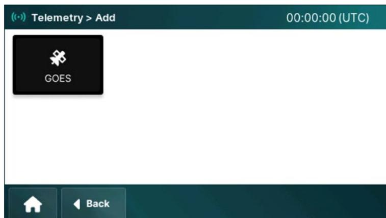
2. Select the telemetry device users wish to add to the data logger by pressing on it. This will navigate users to the configuration screen specific to the selected device to customize its settings.
