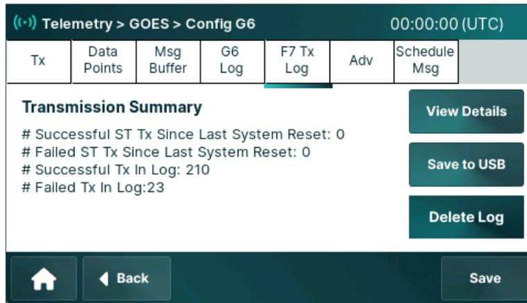
1. The **View Details** button provides access to individual transmission reports. The circular telemetry log file can store approximately 500 reports and will automatically overwrite the oldest entries when the file reaches its capacity.
