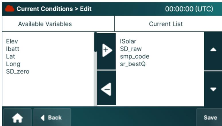
1. Use the **Move Right** and **Move Left Arrow** buttons to transfer data points between the *Available* and *Selected* columns.
