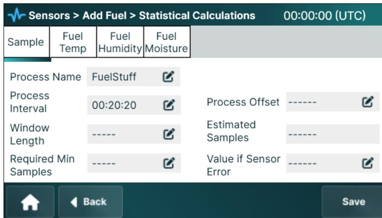
1. **Process Name** displays a default name, which can be modified as needed. The user-defined name helps identify the process when managing multiple statistical calculations.
