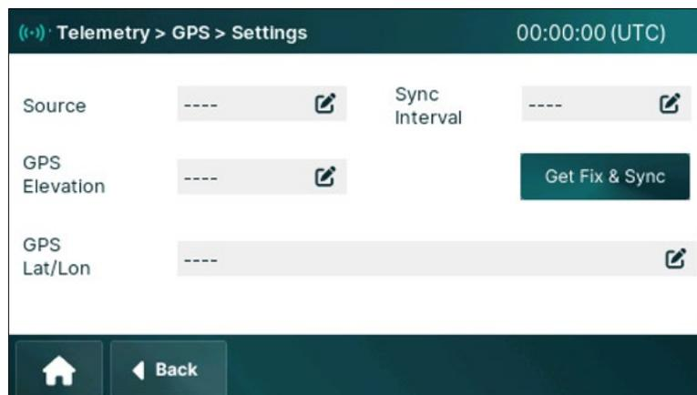
1. **Source** is set to Automate by default to allow the system to select the GPS source automatically.
