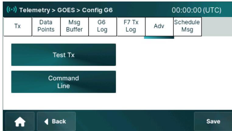
**Test Tx** (Transmission) button configures transmission settings such as NESID, channel, and schedule.
