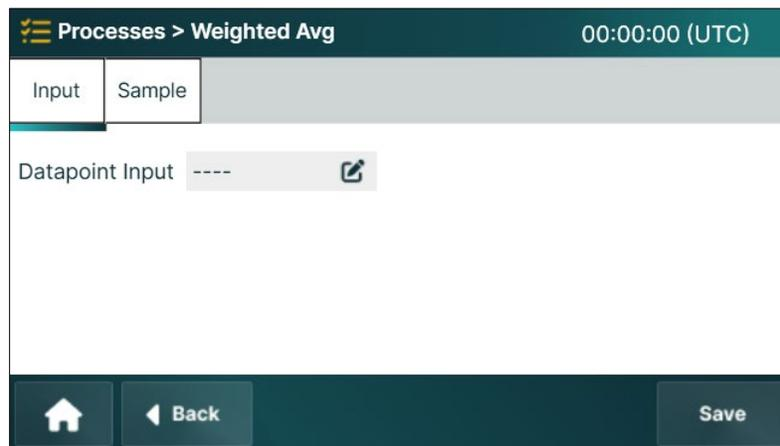
1. Press the **Edit** button to select a data point as an input parameter.
