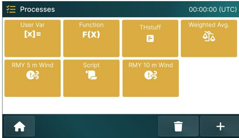
The weighted average function in the data logger is used to smooth out data readings over time, giving more importance (or "weight") to newer readings while still retaining the influence of past data. This helps to filter out sudden spikes or drops in sensor readings, providing a steadier output.
