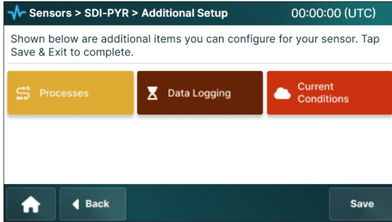
The Processes interface customizes data analysis for the Solar Radiation Sensor, configuring sampling and statistical calculations to provide insights into solar irradiance.
