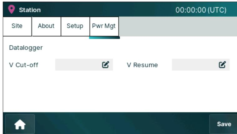
1. Set the ***V Cut-off*** level to define the battery voltage at which the data logger reduces power consumption or shuts down to prevent battery depletion.
