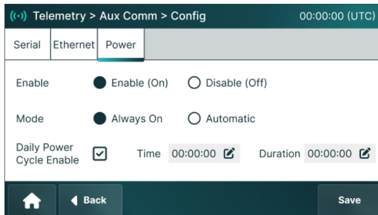
1. Select **Enable** to turn power On or Off for the Aux Comm module.
