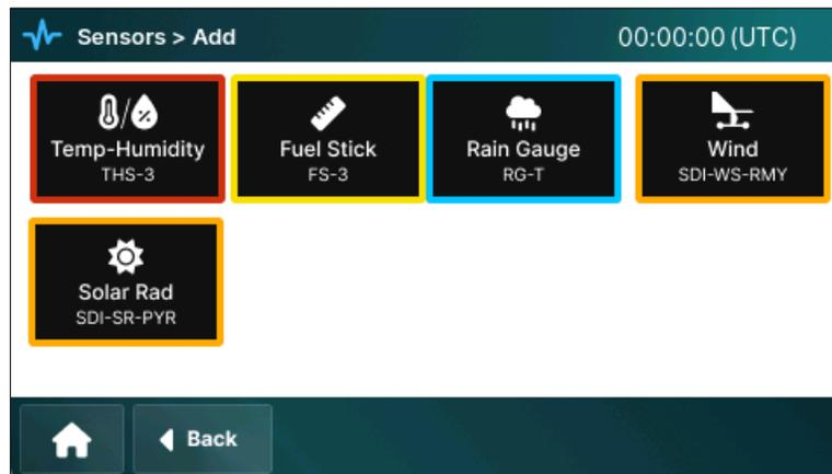
4. Configure sensor using a series of tabbed screen. These set the sensor name, data point names, measurement interval, SDI-12 address, and other sensor-specific operating characteristics.
