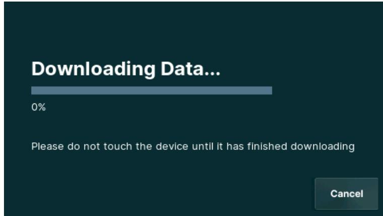
**Note:** Insert a USB flash drive BEFORE selecting Download. Log data extraction and download will not proceed if a USB flash drive is not inserted before starting the download. If this occurs, simply Cancel and reset the format and date range.
