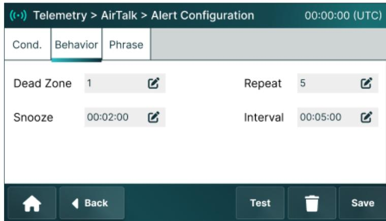
1. **Dead Zone**, also called deadband, neutral zone, or hysteresis, prevents redundant alerts caused by minor data fluctuations.
