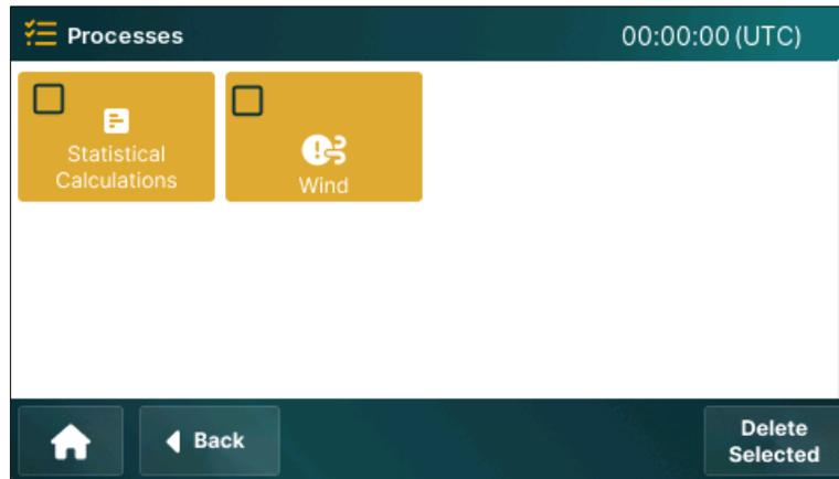
1. Select the checkbox for the desired process/processes users wish to delete.
