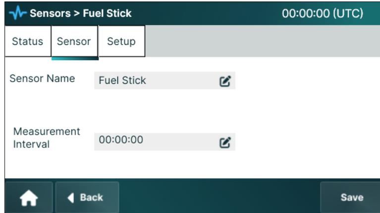
1. **Sensor Name** is pre-set to 'Fuel Stick' and can be modified as required. The user-defined name also appears on the sensor button in the Sensors screen for quick reference.
