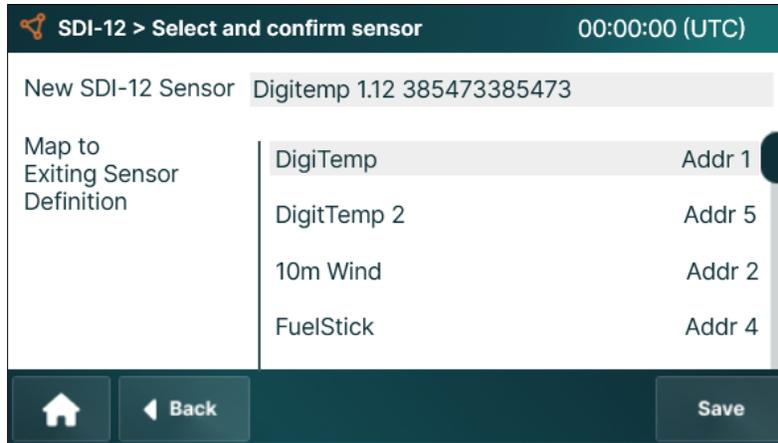
2. From the list, select the defined sensor that matches the address of the new sensor shown at the top of the screen.
