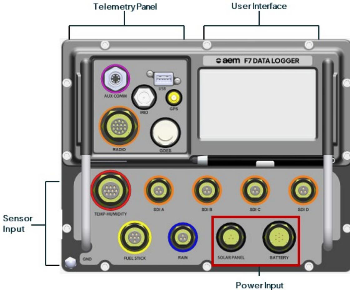
**Note:** H3 is functionally identical to F7, except H3 does not include dedicated Temperature-Humidity or Fuel Stick sensor inputs.
