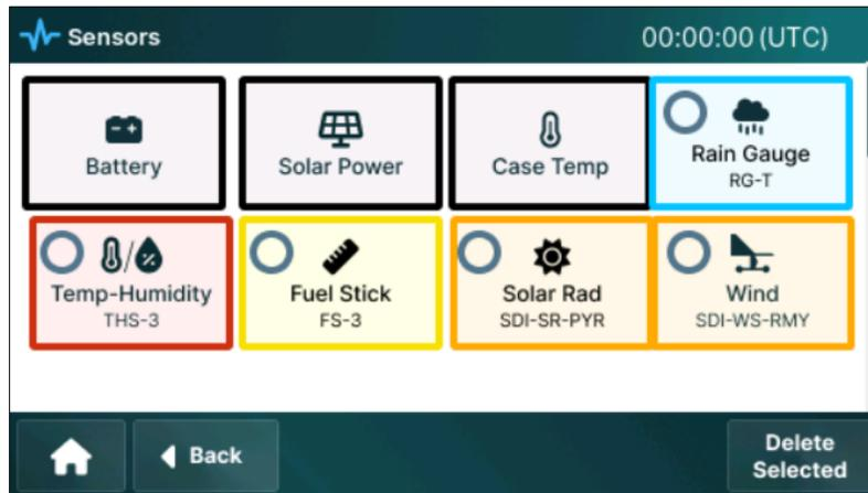
1. On the delete screen, select the check box on the sensor tile.
