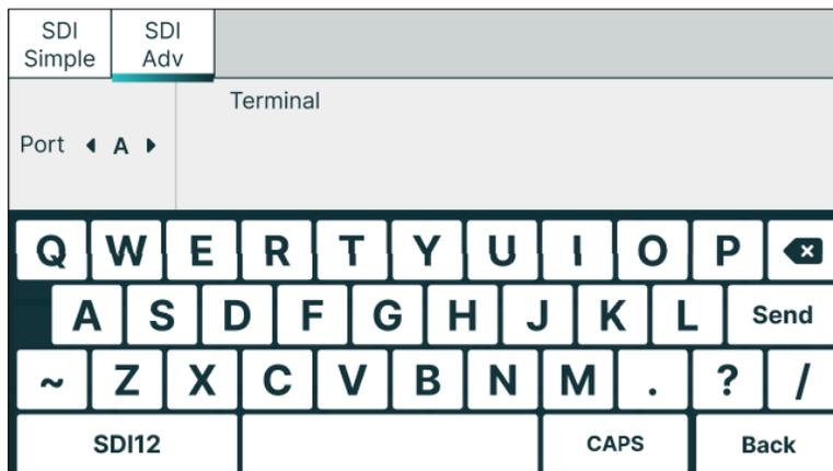
1. Use the arrow buttons to select the SDI *Port*(SDI A, B, C, D) of the connected sensor.
