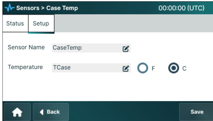
1. **Sensor Name** is pre-set to 'TCase' and can be modified as required. The user-defined name also appears on the sensor tile on the Sensors screen.
