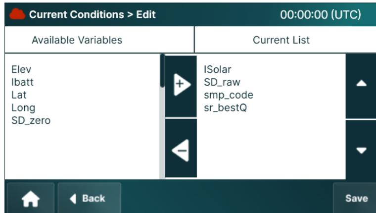
3. Select and move variables from the *Available* to the *Selected* for monitoring. Change the order by selecting the data point and using up and down arrows.
