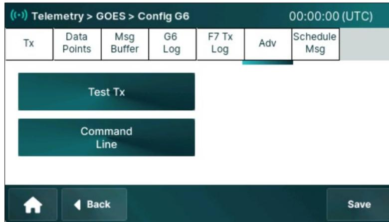
4. Press the **Test Tx** button on the *Config G6* screen. The *Test Tx* screen is displayed.
