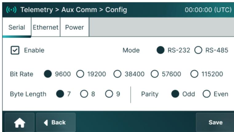
1. Select the **Enable** checkbox to activate serial communication.
