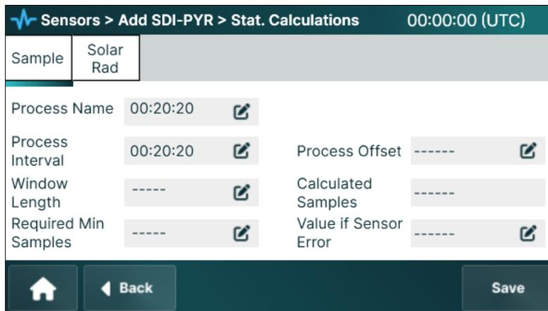
1. *Process Name* is used on the tile that appears on the *Processes* screen.
