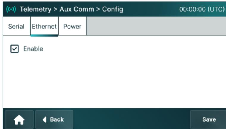
1. Select the **Enable** checkbox to activate Ethernet communication, enabling data transmission over a network.
