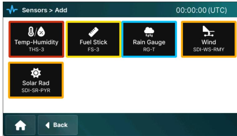
Once a sensor is configured, a new icon appears on the active sensor screen with the sensor name. Users can press the sensor's button to view and edit the associated parameters.
