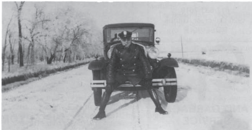
Officer Nestor Pontius and his 1931 Ford Model "A" patrol vehicle. Photo was taken in December of 1933 between Elbow Lake and Herman. Trooper Pontius noted that he could get a top speed of 72 miles per hour with the car's high-compression head and ethyl gasoline. The double-breasted leather jacket was for cold weather and motorcycle duty.
