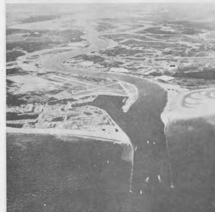
Entrance to Jacksonville Harbor - Jetties protect entrance channel from the Atlantic Ocean into the St. Johns River
