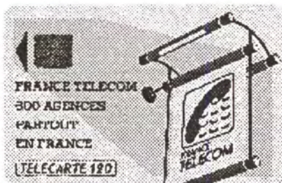
Phone debit cards, such as this one from France, work like computer transit tickets. Each call's cost is deducted from the prepaid card, obviating detailed billing records.
