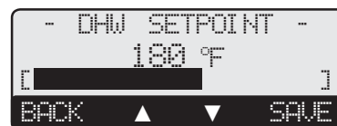
Figure 47. Indirect Domestic Hot Water Setpoint
