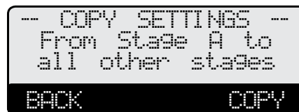
Figure 93. Copy Settings - Boiler A Only
